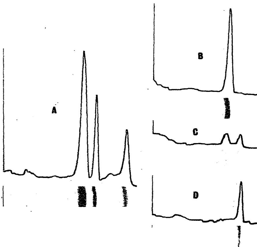
Fig. 2. Electropherograms and scans obtained from a representative fractionation. A = Un-fractionated extract; B = fraction 2; C = fraction 3; D = fraction 4.
